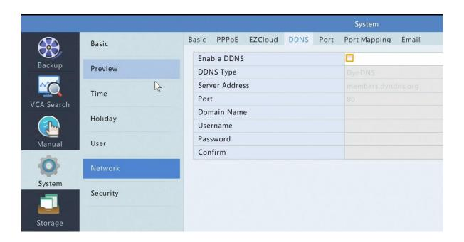
Once within the DDNS section you can now setup your DDNS. To do so select the box next to **Enable DDNS**. Once the box is checked in you will see all of the fields below this option will now be able to be adjusted. You can then select your **DDNS type**. This will be where you will select the service you wish to utilize. These services include: DynDNS, No-IP and EZDDNS. We will be utilizing No-IP in this case.
