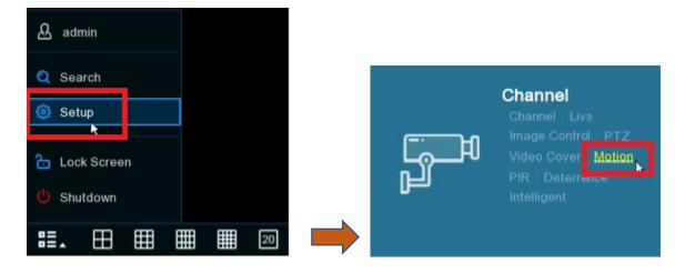
**Step 2)** Select the gear icon under the tab labeled **"setup"** for any channel you'd like to configure.
