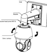
Step 6: After rotating the dome camera to the proper position, tighten the 2 socket head cap screws M6\*16 on the bracket.
