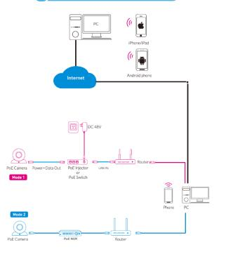
Attention: There are two connection modes: 1. For non-PoE router,pls connect the camera by a PoE switch or a PoE injector. 2. For a POE NVR, pls connect the camera directly to the POE NVR, then follow the below steps.
