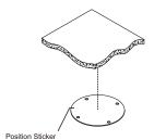
Apply the position sticker to the desired camera mounting position.
