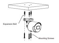
Insert three expansion bolts in place into the ceiling and fix the equipment with three mounting screws.
