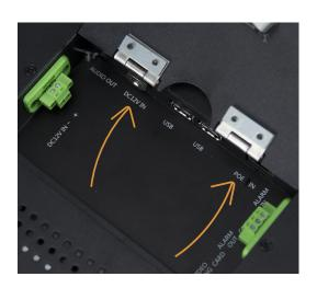
Ports are located via back of device behind lock door.
